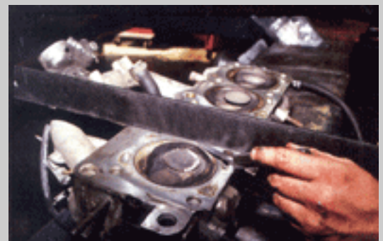
Fig 1. Check with a feeler gauge for warping between the surface and the straightedge.
